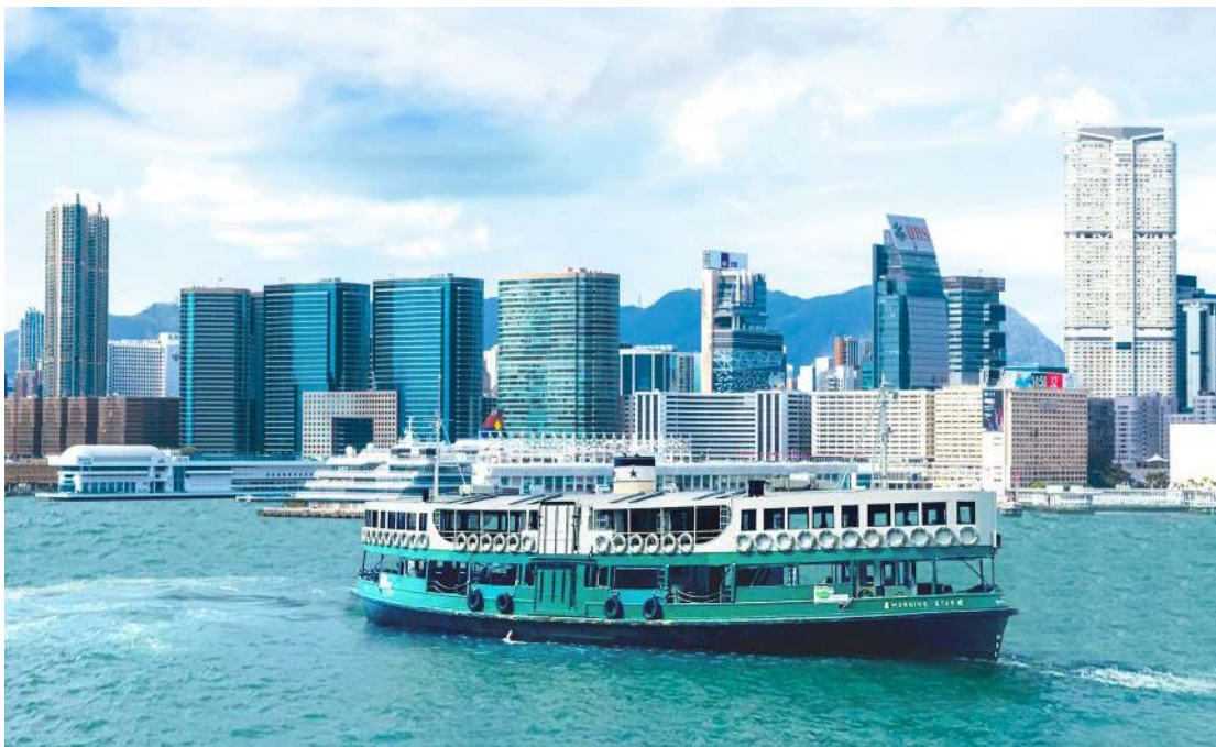
3. "Morning Star", equipped with diesel-electric propulsion system, becomes the first low emission green ferry running daily service in Hong Kong.
